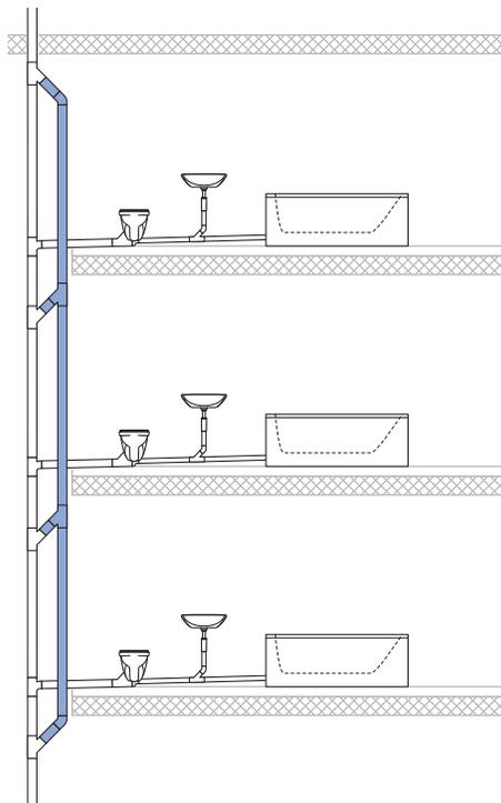
Figure 36: Secondary ventilation pipe
