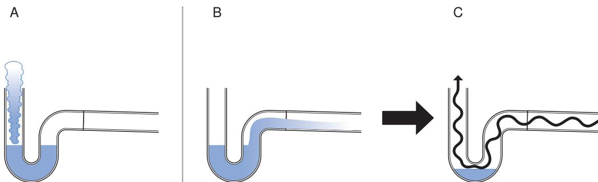
Figure 29: Causes which reduce the water seal depth
