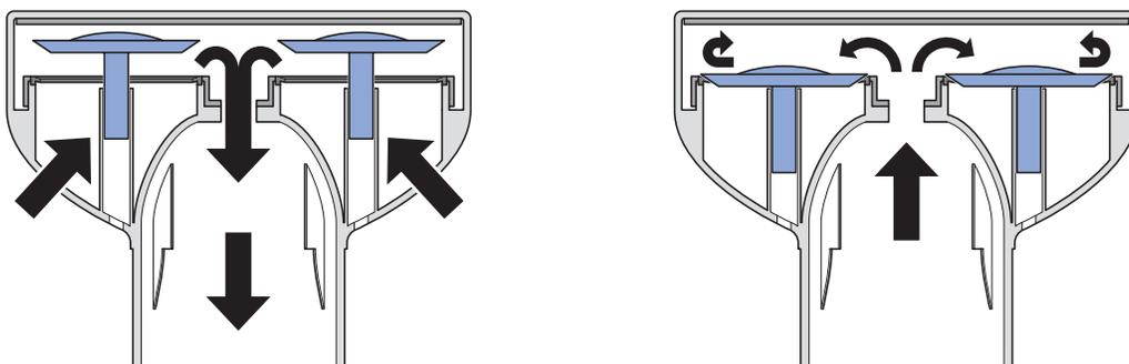
Figure 39: Open and closed air admittance valve
