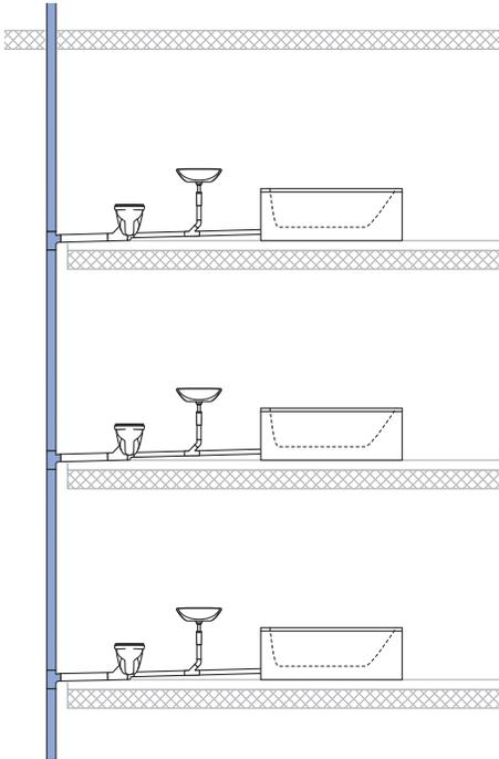
Figure 35: Main ventilation pipe
