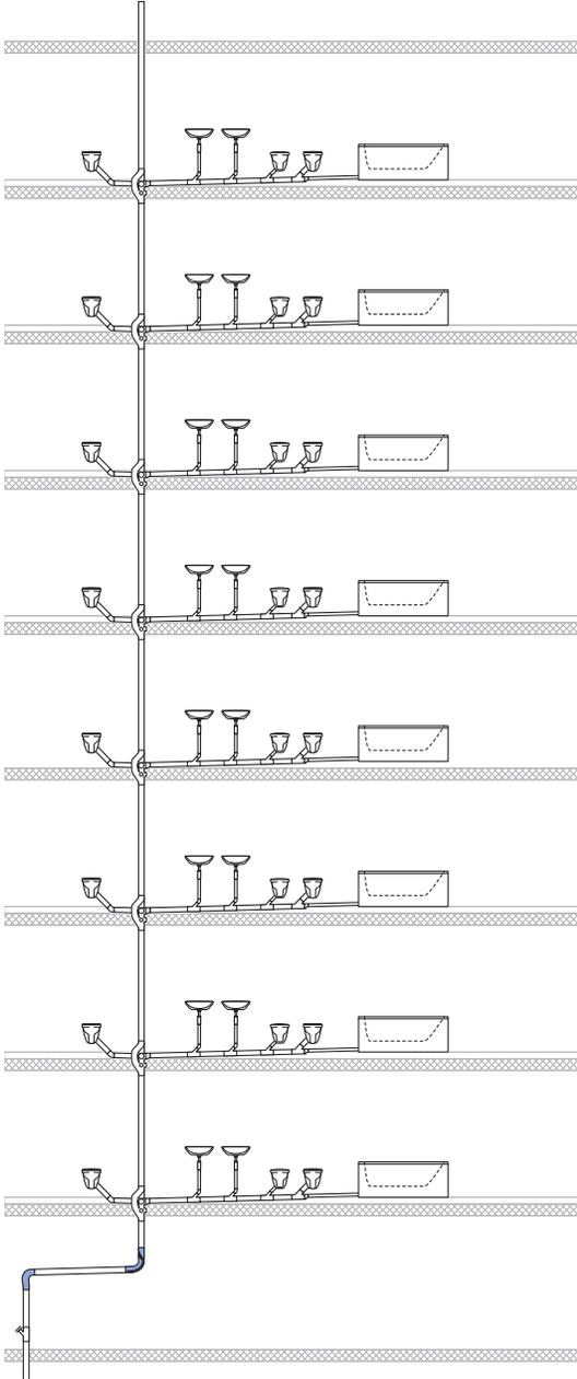
Figure 69: Drainage system with Geberit SuperTube
