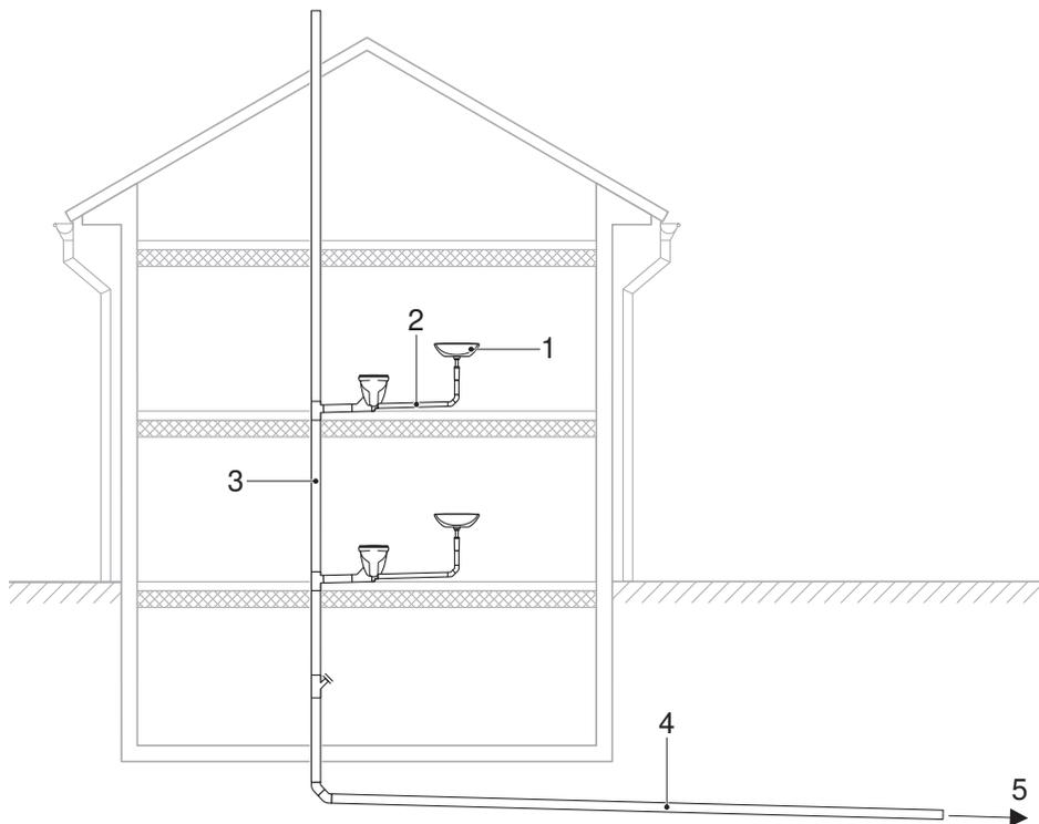
Figure 10: Basic structure of a building drainage system
