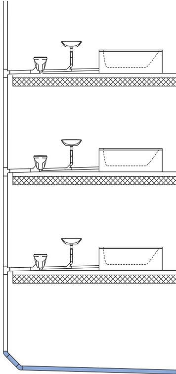
Figure 33: Underground and collector pipe
