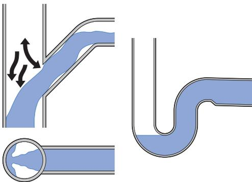
Figure 50: Flow conditions in an equal and reduced branch fitting 45° in the stack
