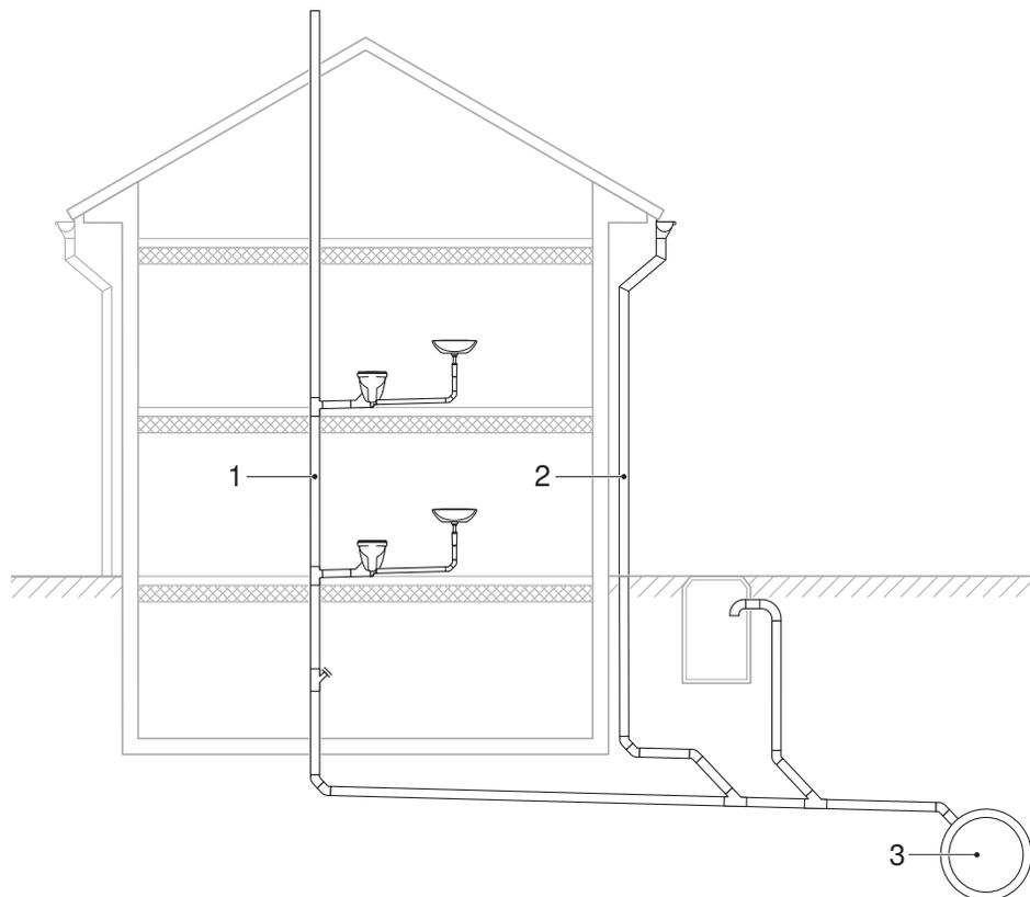
Figure 12: Structure of a combined system
