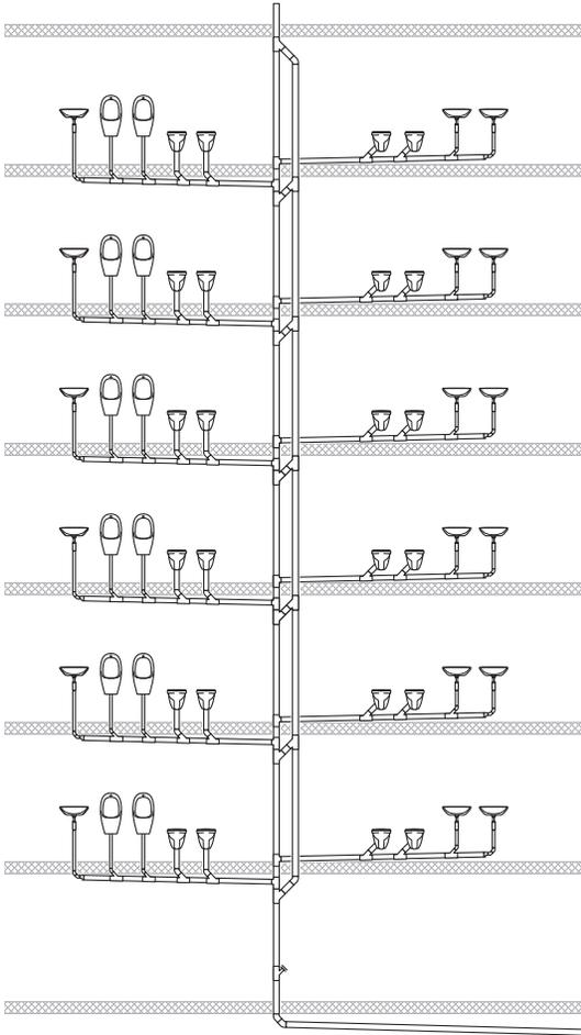
Figure 65: Drainage system with direct secondary ventilation
