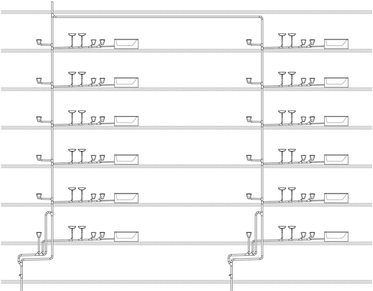
Figure 64: Drainage system with collective ventilation
