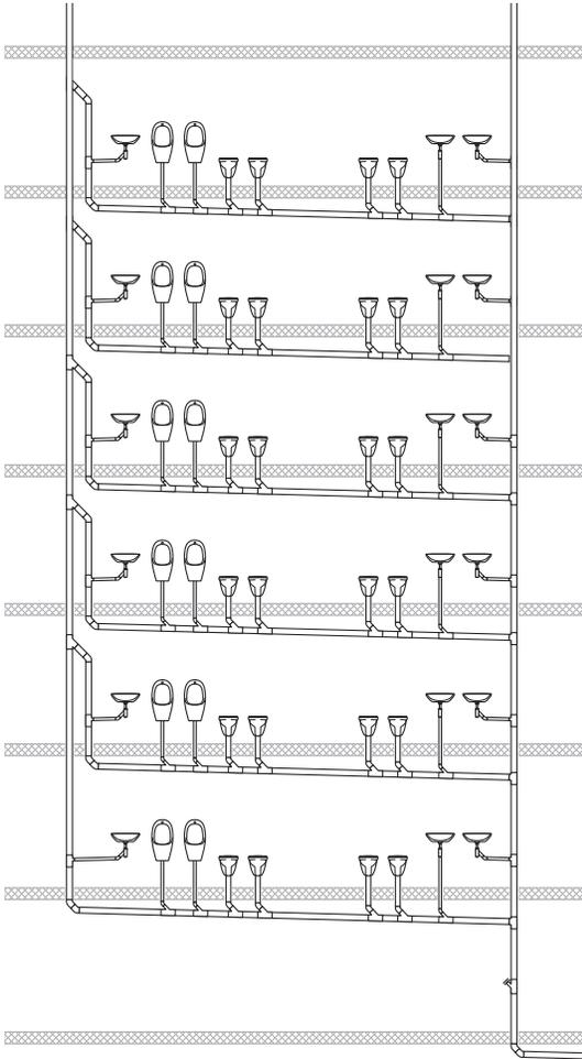
Figure 66: Drainage system with indirect secondary ventilation
