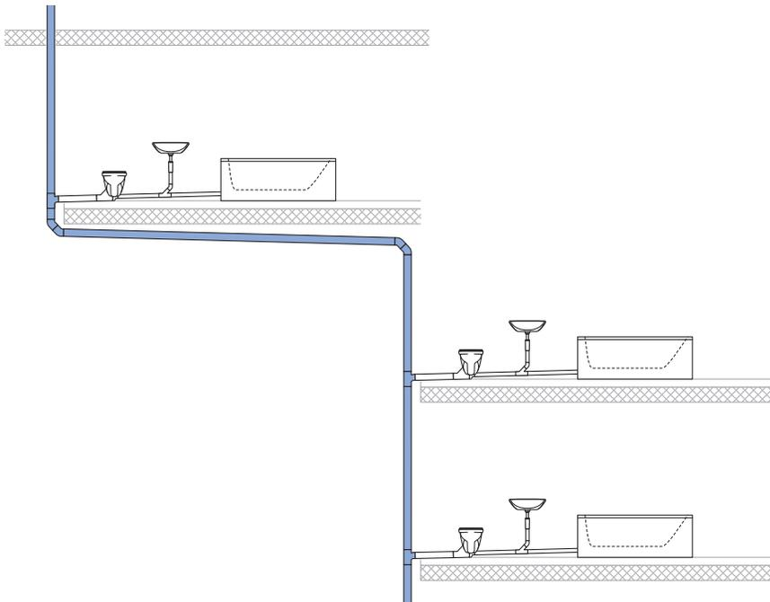
Figure 32: Stack with stack offset
