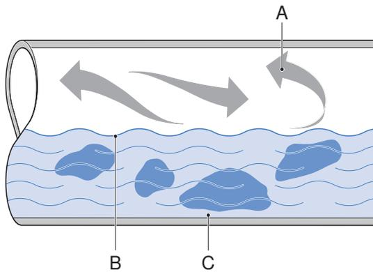
Figure 15: Flow conditions in horizontal pipe sections
