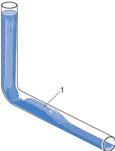
Figure 41: Waste water splashes up the sides of the pipe after a direction change in a bend  $90^\circ$
