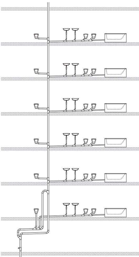
Figure 63: Drainage system with individual ventilation
