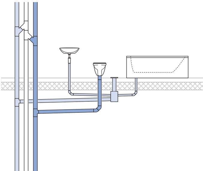
Figure 71: Laying the branch discharge pipe under the ceiling, three stacks
